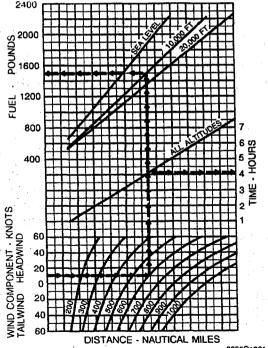
Figure 5-34. Fuel And Time Required - Maximum Range Power (Sheet 2 of 2)
