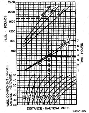
Figure 5-18. Fuel And Time Required - Maximum Cruise Power (Sheet 2 of 2)
