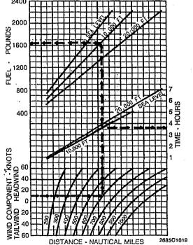
Figure 5-33. Fuel And Time Required - Maximum Cruise Power (Sheet 2 of 2)
