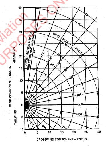
Figure 5-7. Wind Components
