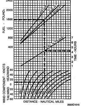
Figure 5-19. Fuel And Time Required - Maximum Range Power (Sheet 2 of 2)
