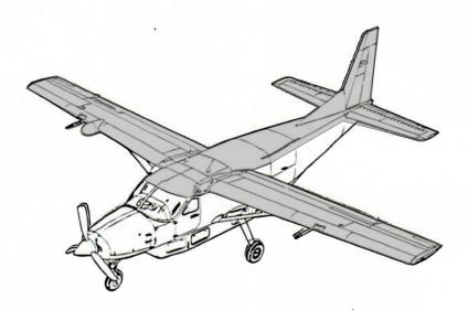
NOTE: ANTI-ICE FLUID SHOULD BE APPLIED AT LOW PRESSURE TO FORM A THIN FILM ON SURFACES. FLUID SHOULD JUST COVER AIRPLANE WITHOUT RUNOFF.
