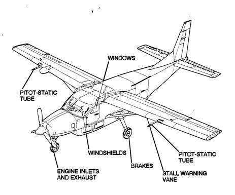
DIRECT SPRAY AVOIDANCE AREAS: ENGINE INLETS AND EXHAUST, BRAKES, PITOT STATIC TUBES, WINDSHIELDS, CABIN WINDOWS, AND STALL WARNING VANE.
