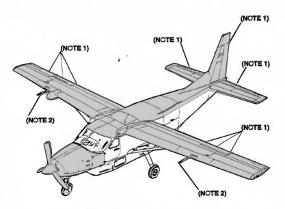
NOTE 1: GIVE SPECIAL ATTENTION TO THE GAPS BETWEEN THE FLIGHT CONTROLS. ALL SNOW, ICE AND SLUSH MUST BE REMOVED FROM THESE GAPS.
